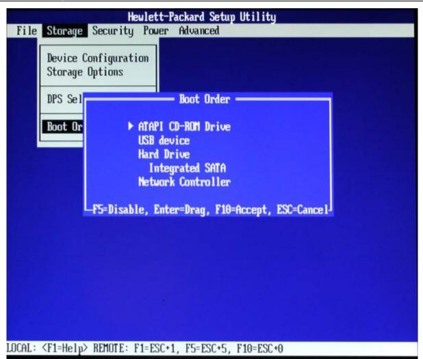
We will be booting from a USB stick, so let's move the USB device to the top by pressing Enter, then the up arrow.
